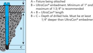
maximum of 1-3/4" is recommended  $A + B = UltraCon^{\otimes} length$ B + C = Depth of drilled hole. Must be at least 1/4" deeper than UltraCon® embedment
