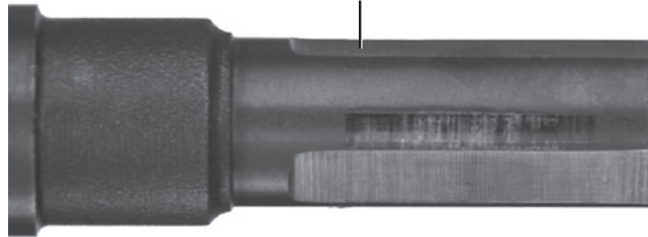
Damage caused by the drill chuck jaws resting on the shank as opposed to resting on the driving flats
