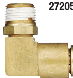
Male Elbow Swivel 360° 3/8 Tube x 1/4 NPT
