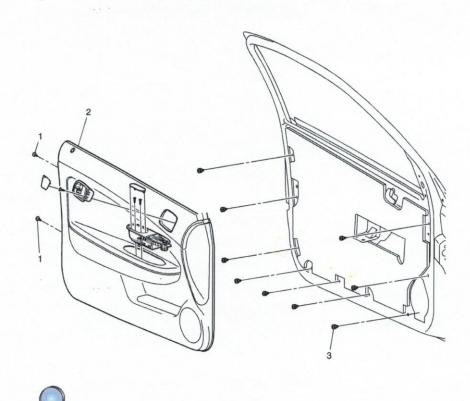
1. Remove the front driver side door trim panel. Refer to Front Side Door Trim Panel Replacement in SI.
