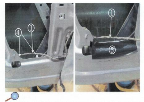
6. Apply a 114 mm (4.5 in) piece of Scotch Electrical Moisture Sealant Tape, P/N 06147 or equivalent (5) to metal edge of the door (4) as shown in the photograph.
