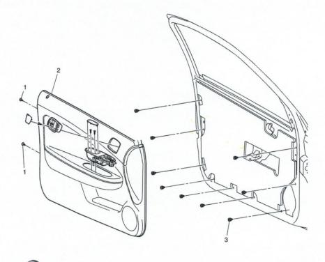
Install the front driver side door trim panel. Refer to Front Side Door Trim Panel Replacement in SI.
