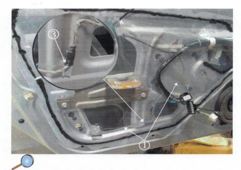
If the SIS wire harness clip is positioned in the vertical position (3), partially remove the vapor barrier to gain access to the SIS wiring harness and clip. Remove the pull cup bracket to partially remove the vapor barrier. Proceed to step 4.
